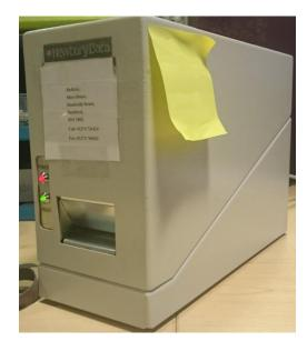
On ND4800 series printers, there is a power button on the front which sets the printer to standby mode.
